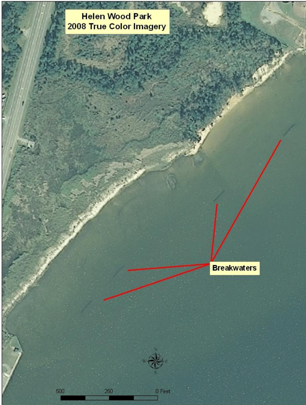
Figure 5. Aerial of Helen Wood Park breakwaters provided by ADCNR-State Lands Division. Treatments visible from North to South are North Oyster, North Reef Ball, South Oyster, South Reef Ball. North control is located between the visible breakwaters, and South Control is just North of the two southernmost breakwaters.
