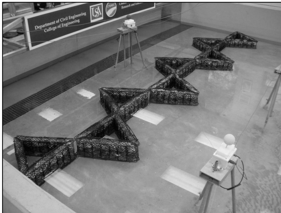
Figure 9: The University of South Alabama wave basin setup for conducting the experimental testing of the ReefBLK SM units.
