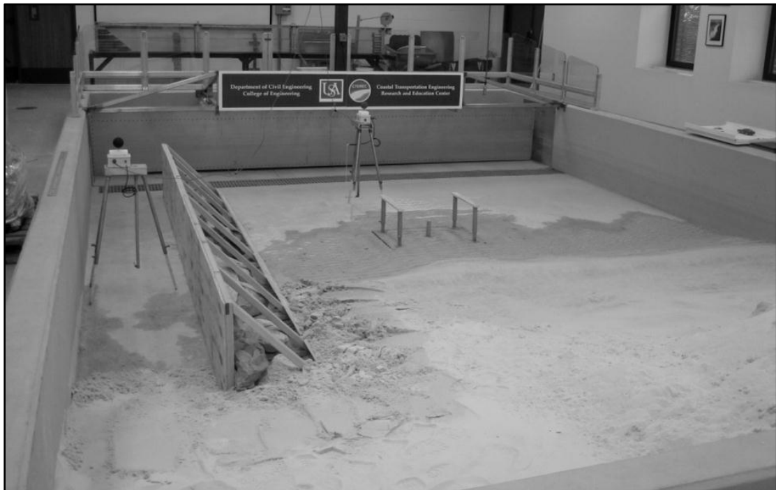
Figure 1: University of South Alabama wave basin with splitter wall installed and graded beach face in preparation for testing the bagged oyster shell.
