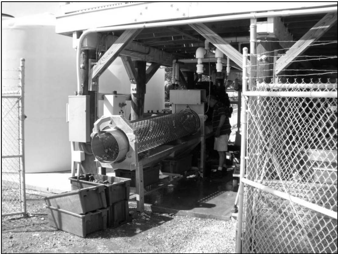
Figure 14: Oyster shell being processed through the Chesapeake Bay Oyster Company sorter at the Auburn Shellfish Laboratory.
