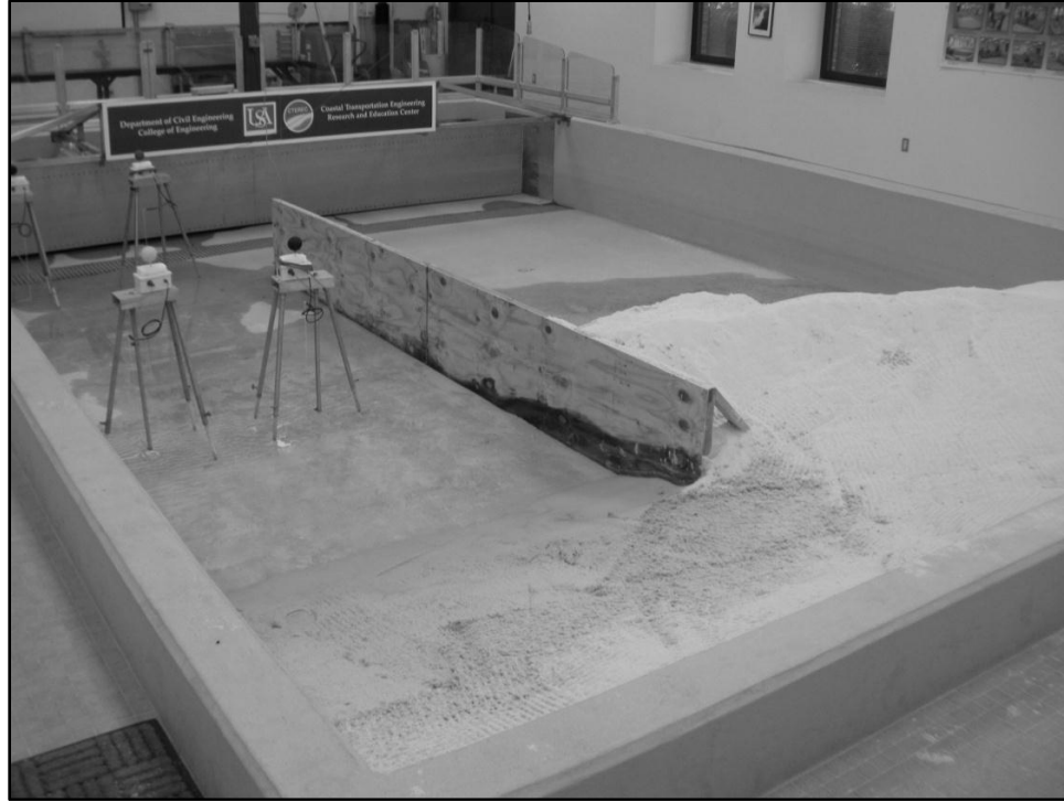
Figure 5: University of South Alabama wave basin setup for conducting experimental testing of the concrete pyramids.
