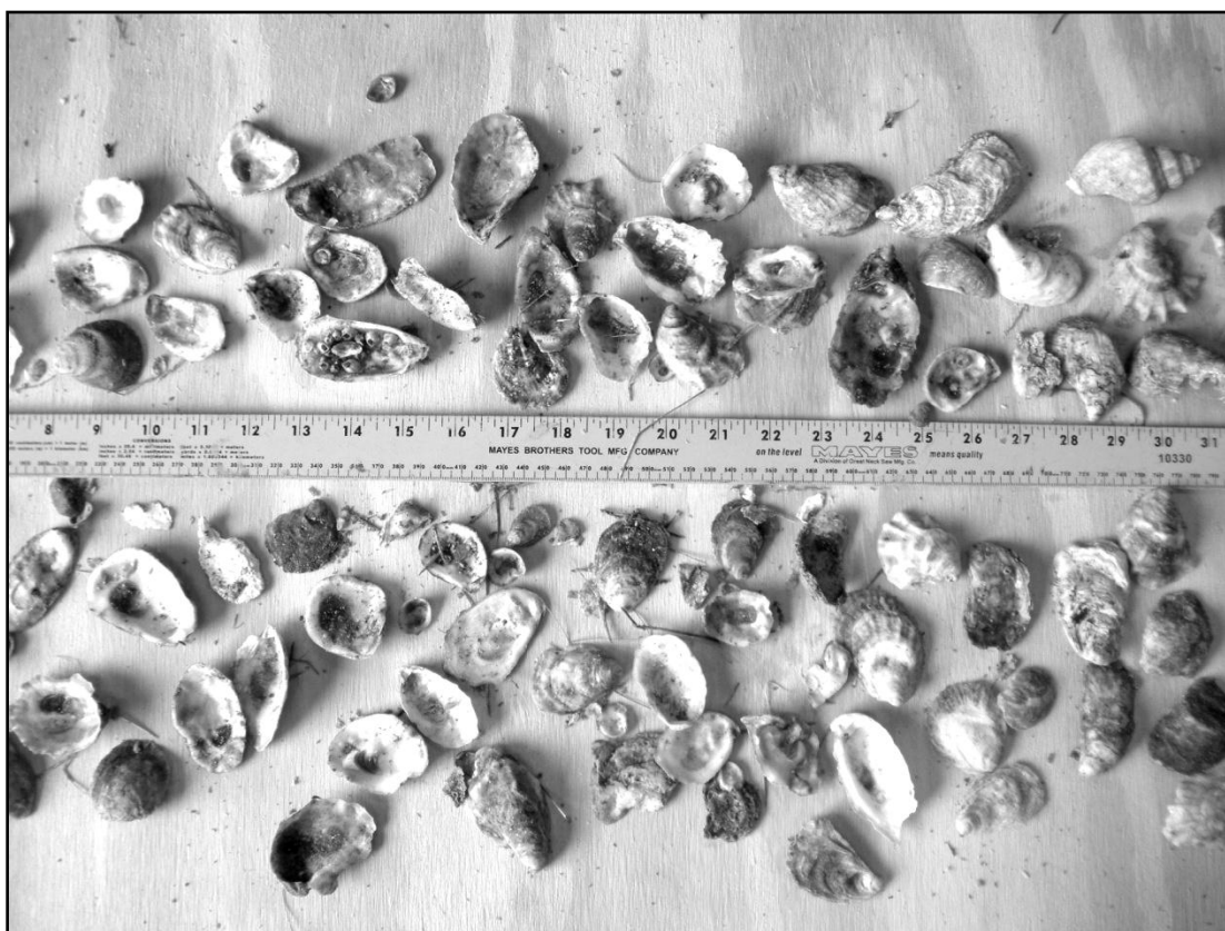
Figure A5: Oyster shell distribution with scale used in the ReefBLK SM construction.
