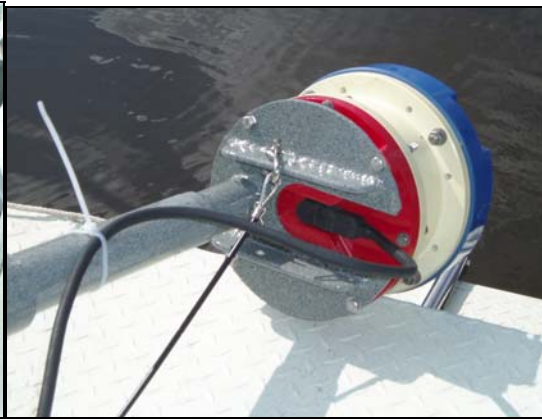
Figure 7. ADCP with custom mount.
