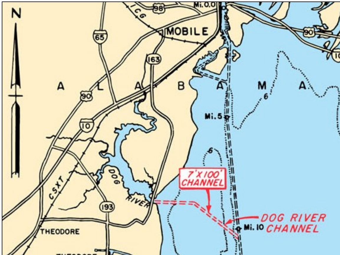
Figure 6. Hydrologic Modification through Channel Dredging (USACE 2008).
