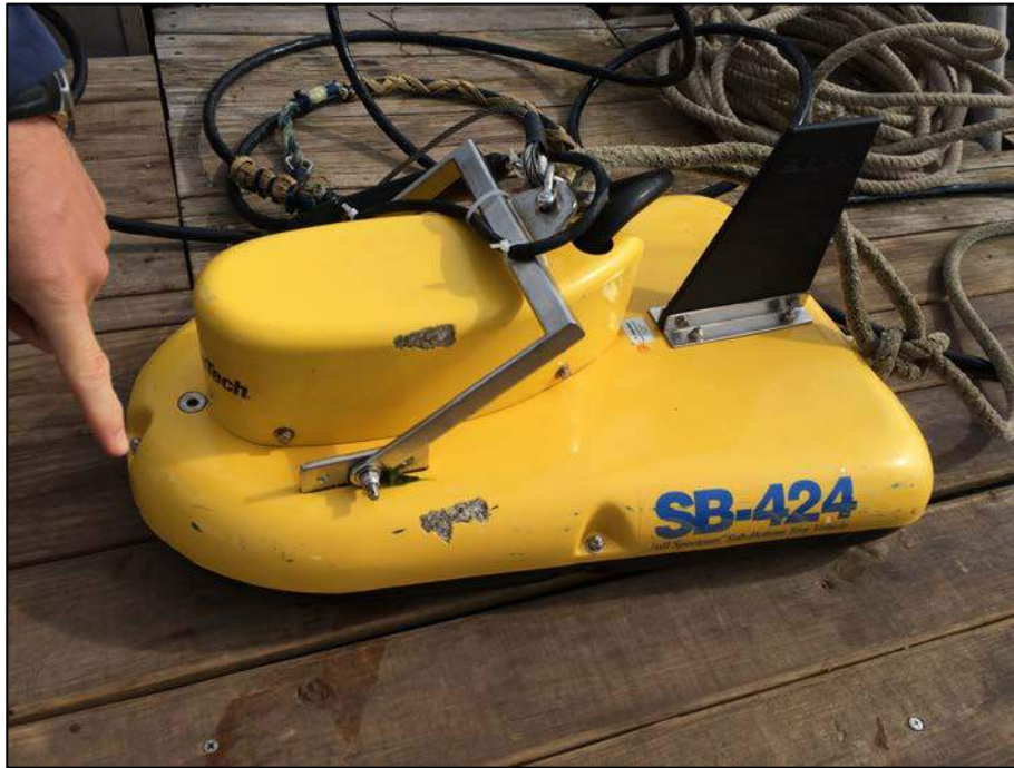
Figure 3-08. The EdgeTech SB-424 towfish employed during the survey.
