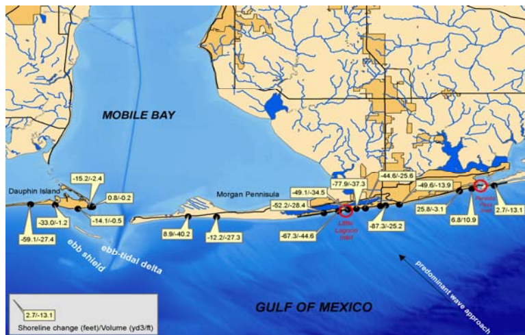
Figure 10: Results from BMAP V2 using 2004 and post-Hurricane Ivan cross-shore profile data to convey shoreline and net volume changes.
