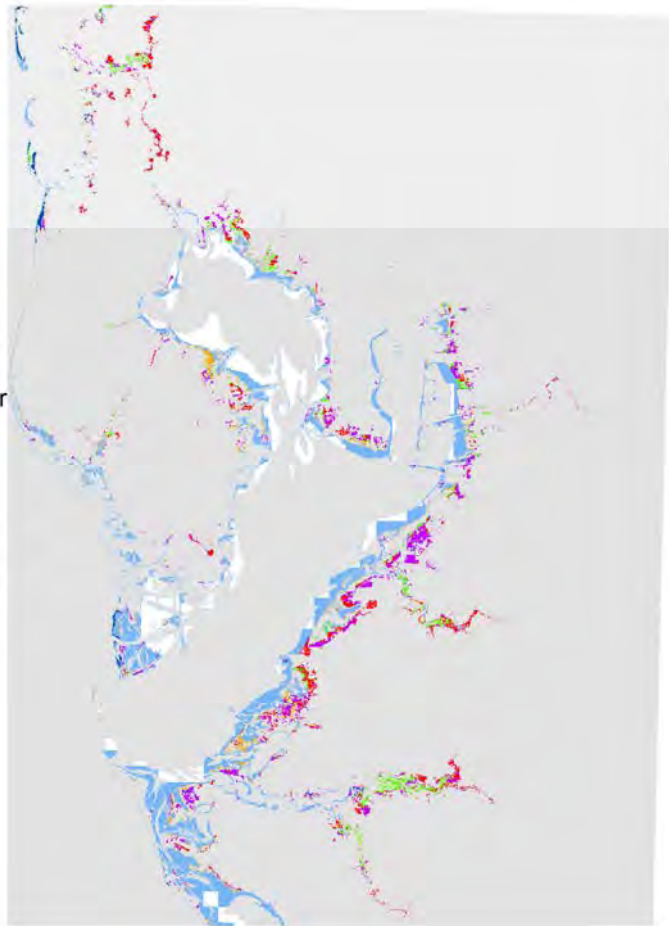
Figure 45. Tampa Bay Study Area SLAMM results - change in coastal wetland cover under a 1 meter SLR scenario, developed dry land protected from changing.
