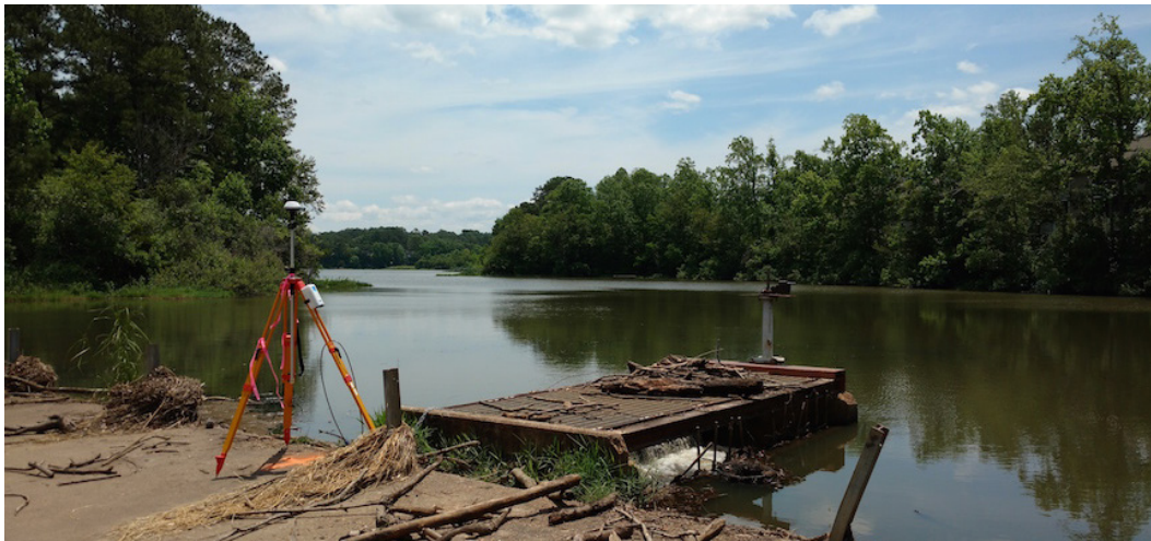
Figure 5. The RTK base station location used for the bathymetric mapping.
