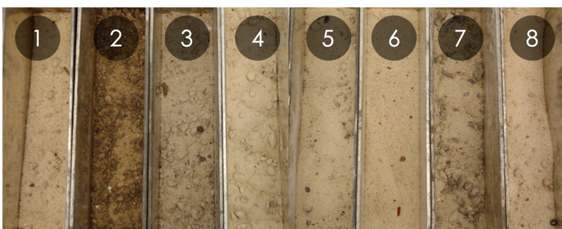
Figure B- 3. Oven and air dried sediment core samples (numbering is LF00x).
