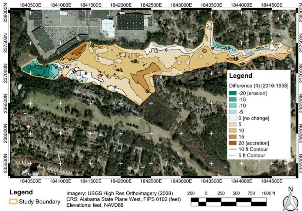
Figure 15. Elevation differences between 1958 and 2016. Positive values (browns) represent shoaling or shallowing of the lake. The negative values (greens) indicate areas where the lake has deepened since 1958.
