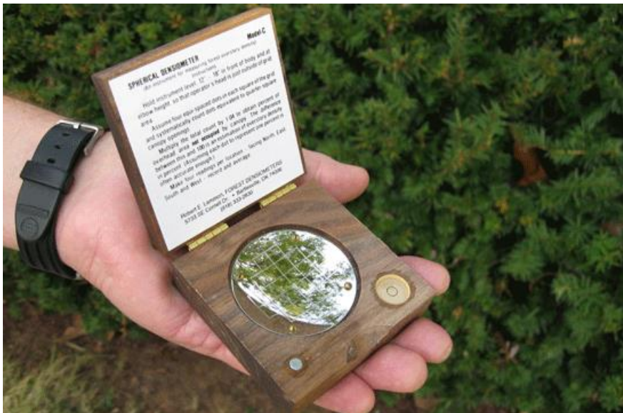
Figure 14: Image of the densiometer instrument. Canopy cover is determined using the gridded mirror and presence/ absence within the grid. ii
