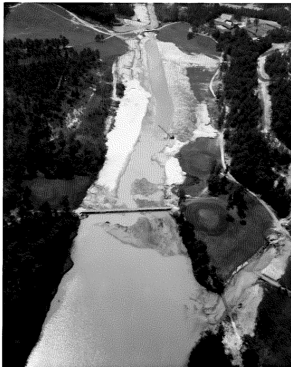
Fig. 12.--View looking up southeastern arm of Lake Forest reservoir where Tiawasee Creek enters lake. Note extensive deposition along banks (S. Coleman photo, 1979).
