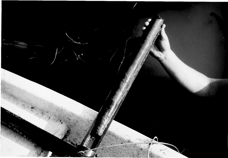
Fig. 14.--"Split spoon" core of typical clay-rich sediments in D'Olive Bay.
