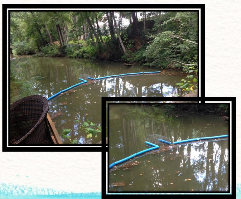
Purpose – Create a solution for small stream litter collection from stormwater runoff to enhance water quality and aesthetics throughout a watershed.
