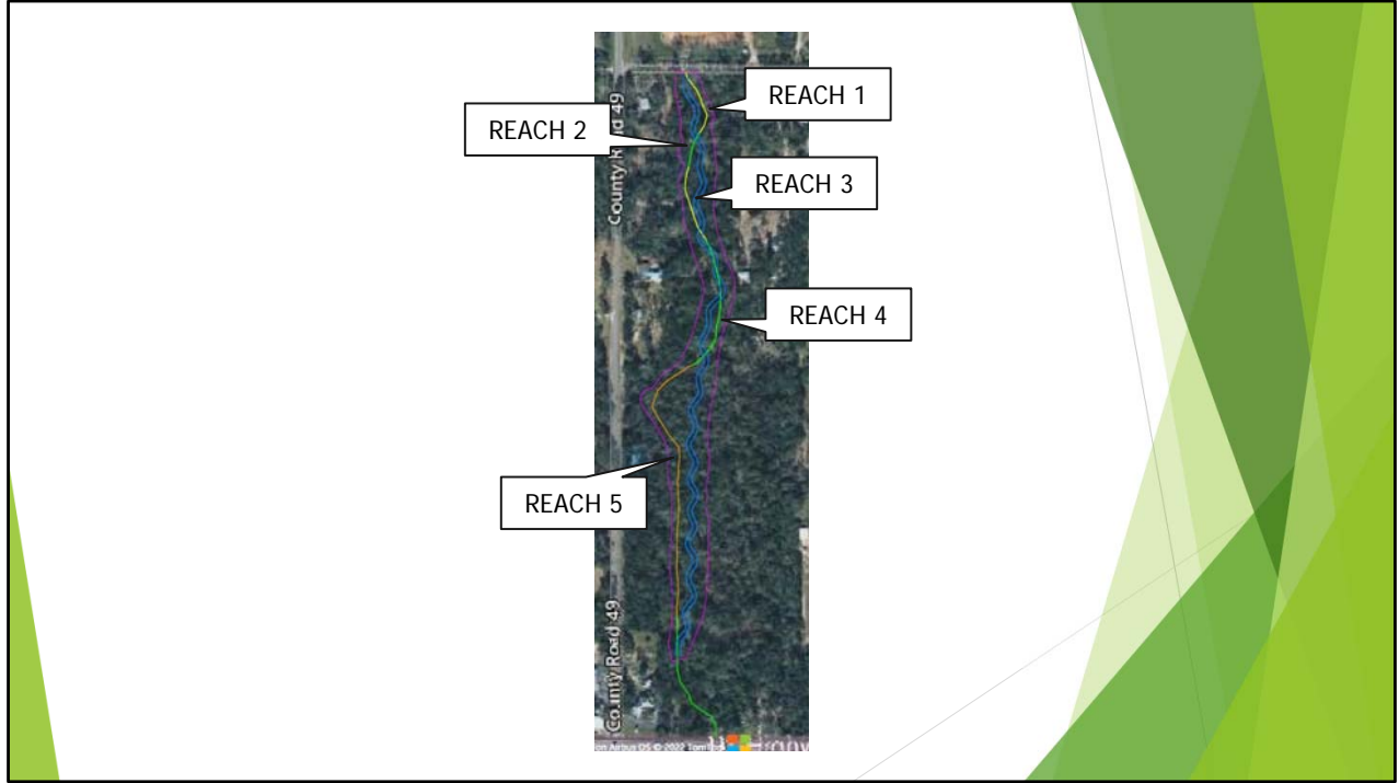
An unnamed tributary between Beasley Road and HWY 98 is targeted for restoration. Reach 5 appears to be the primary area of instability, totaling about 1,125 linear feet.
