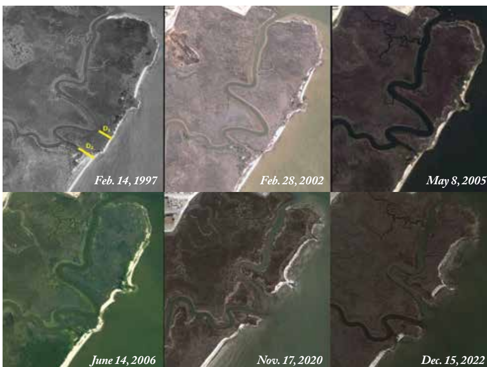
A sequence of satellite images documenting the progressive and dramatic deterioration of the marsh shoreline from 1997 until December 2022, totaling 51 acres lost to date.
