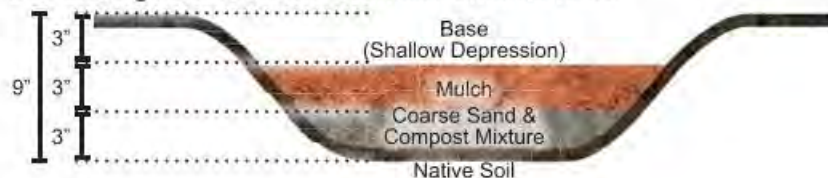
Figure 7.6 Rain Garden Excavation Depths
