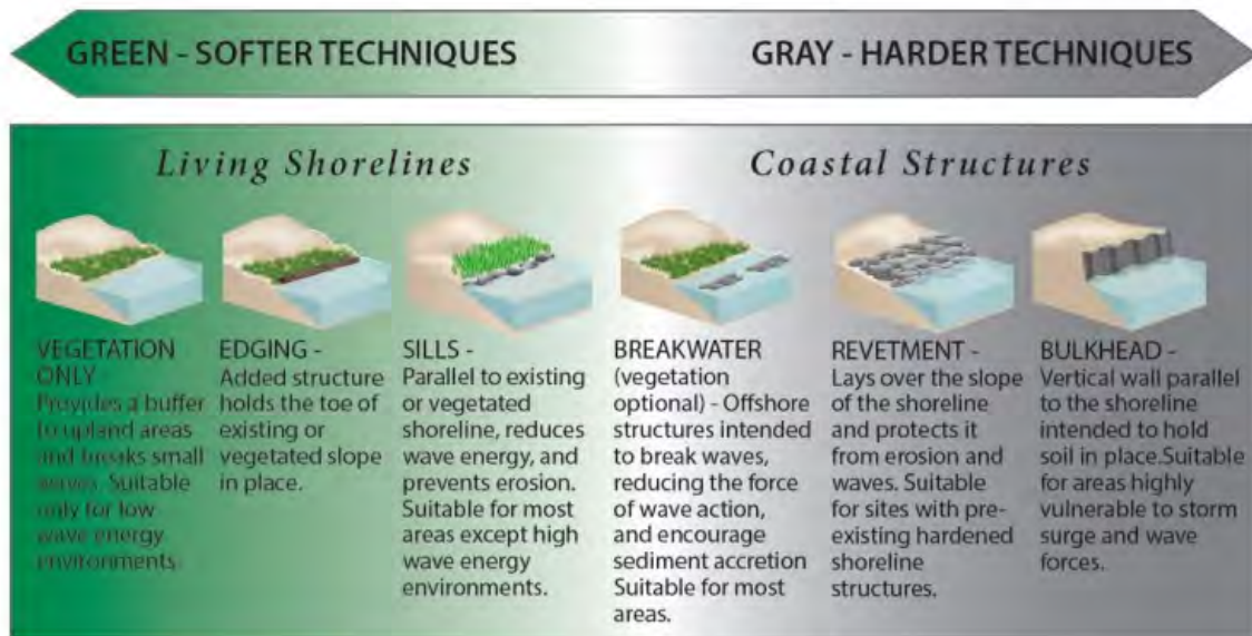
Figure 7.14 Green (soft) to gray (hard) shoreline stabilization techniques
