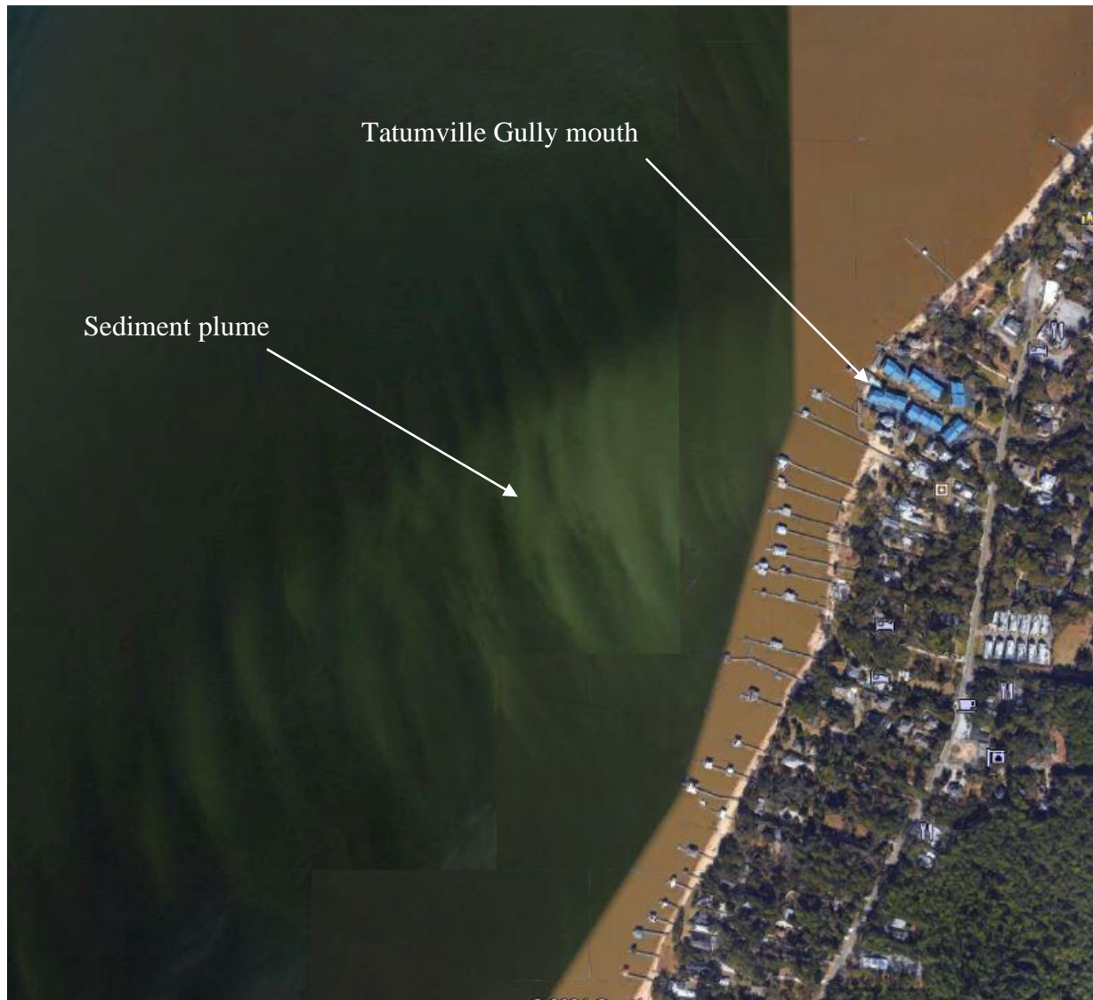
Figure 22.—Sediment plume shown on 1985 satellite imagery, extending southwestward into Mobile Bay from the mouth of Tatumville Gully (Google Earth, 2020).
