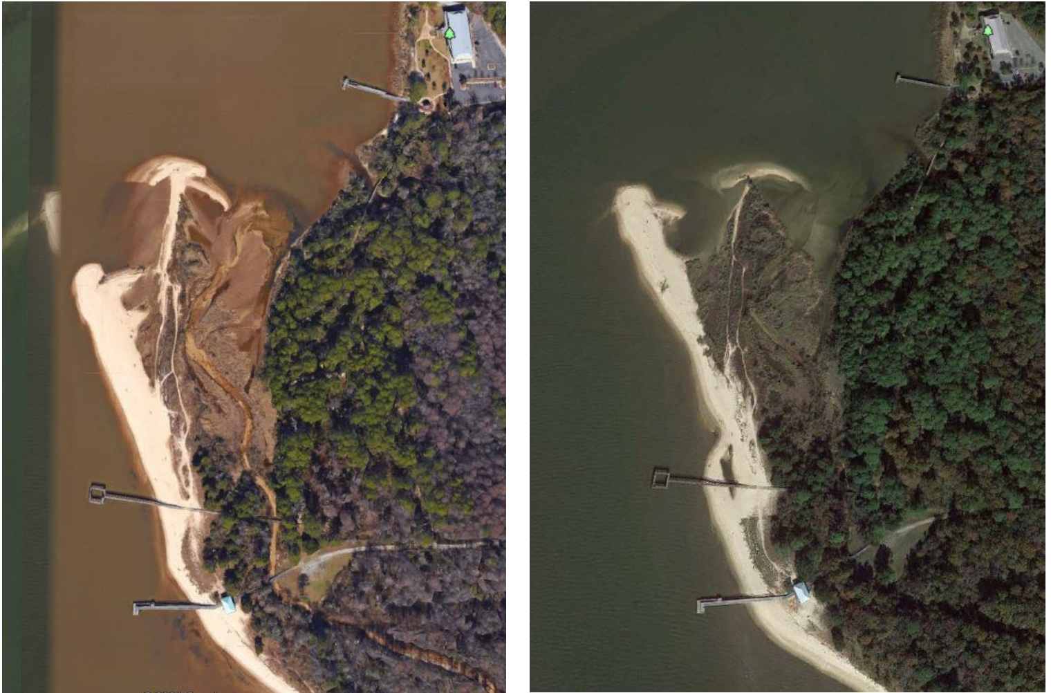
Figure 17.—Sediment deposition into D'Olive Bay at the mouth of Yancey Branch in 1985(left) and 2019 (right) (Google Earth, 2020).
