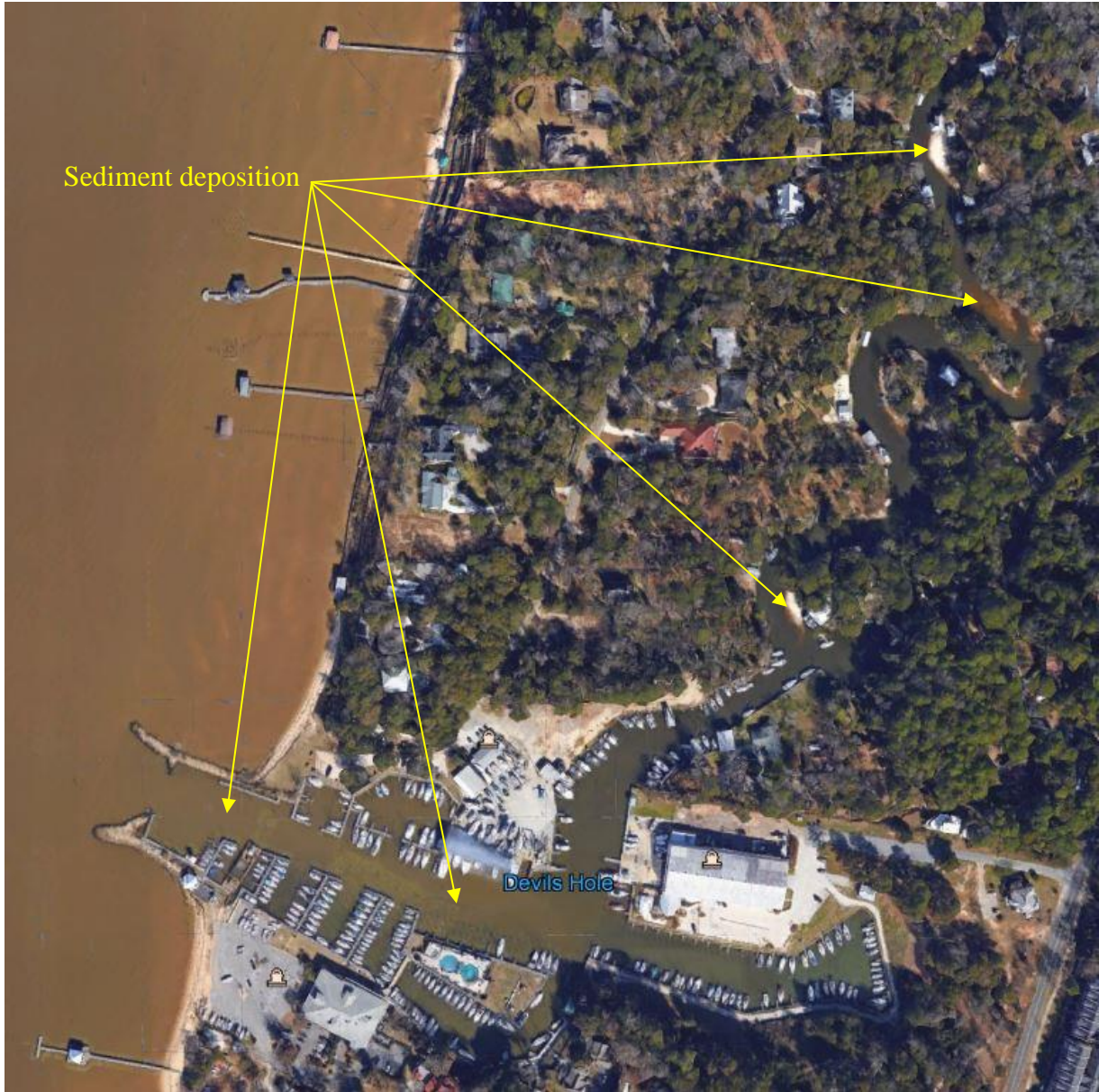
Figure 19.—Sediment deposition in the tidally influenced reach and yacht basin of Fly Creek in 1985 (Google Earth, 2020).
