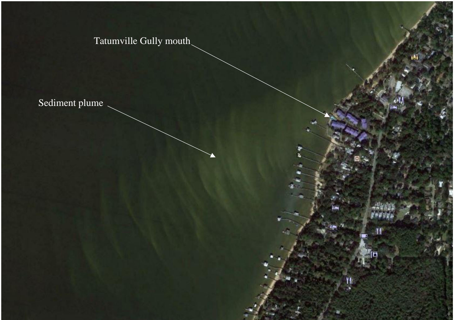
Figure 24.—Sediment plume from the mouth of Tatumville Gully shown on 2019 satellite imagery (Google Earth, 2020).
