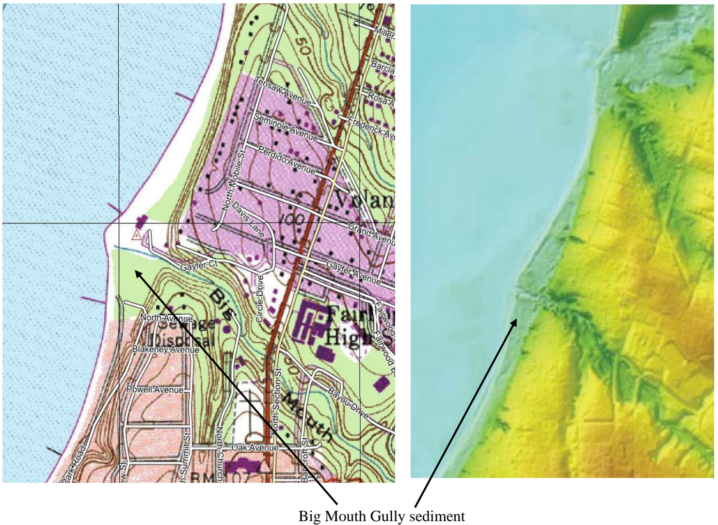
Figure 21.—USGS topographic and topobathymetric maps, showing sediment deposition at the mouth of Big Mouth Gully.
