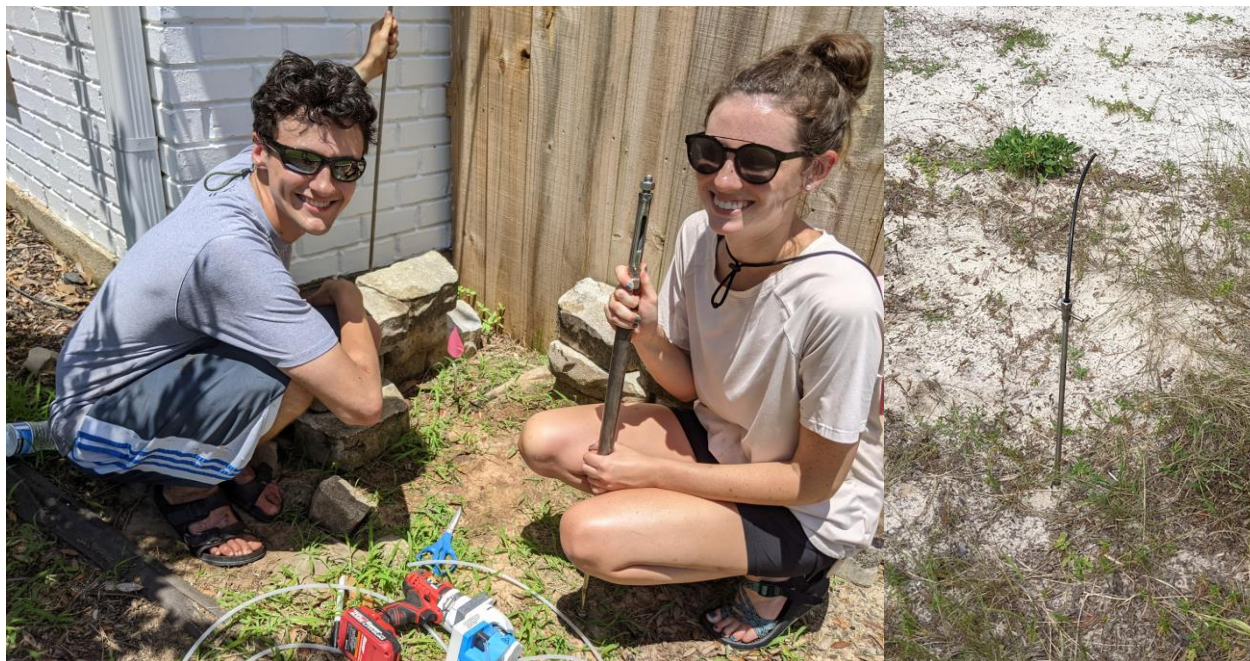
Figure 8 – (Left) USA researchers pose with the piezometer installation rod, slide hammer, and peristaltic pump. The planted polyethylene piezometer (small tube) is located just below the pink flag in the center of the picture. (Right) Polyethylene piezometer and steel installation rod shortly after planting with slide hammer.
