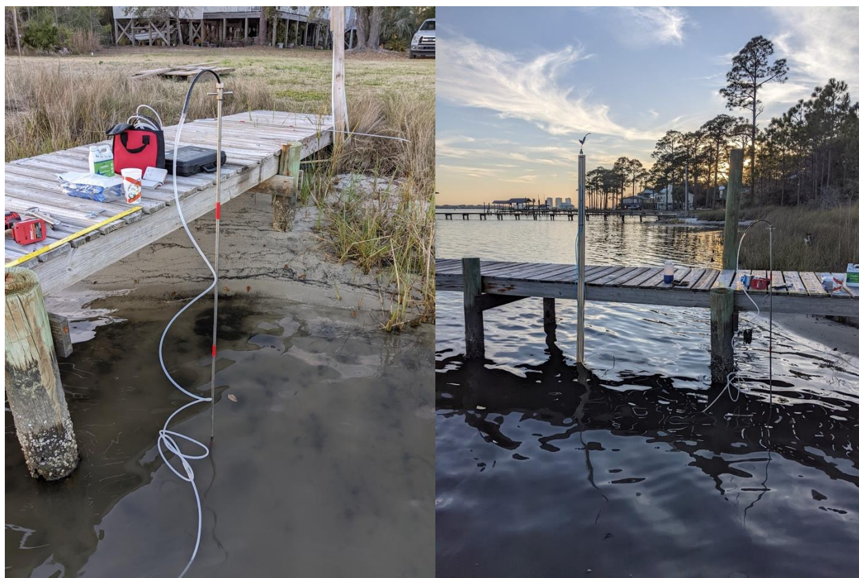
Figure 24 – SedPoint apparatus used for sampling the subterranean estuary. There was no evidence of terrestrial submarine groundwater discharge during spring 2022, and conditions were generally reducing and slightly acidic, not unlike the inland aquifer.
